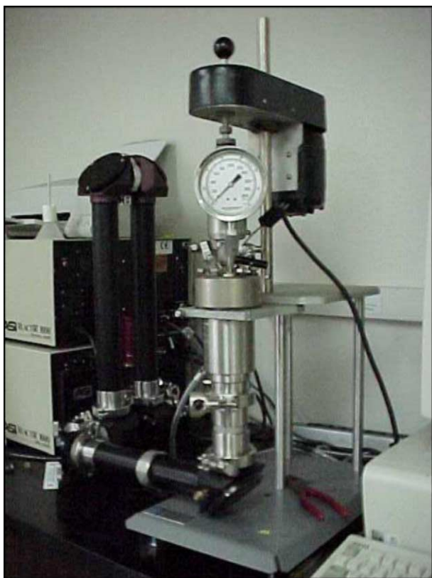
Fig. 3. ASI ® ReactIR 1000 reaction analysis system with stainless steel Parr ® autoclave modified with a permanently mounted ATR crystal (SiComp) at the bottom of the reactor (purchased from Mettler Toledo).
