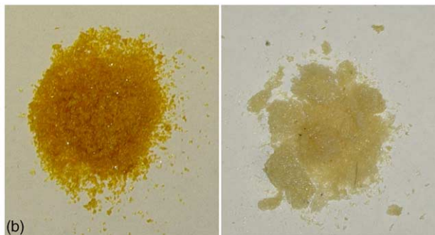
Fig. 9. (a) In situ infrared spectra of TMSO polycarbonate dissolved in epoxide/CO 2 and liquid CO 2 . (b) Photos of TMSO polycarbonate before (left) and after (right) dissolution in liquid CO 2 .
